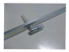
5) Gently pull the silicone tube to near the valve to spacer bar:
