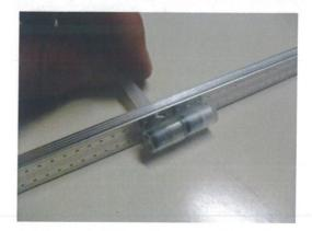
WARNING: BE SURE THE TWO-WAY VALVE HAS BEEN ASSEMBLED PROPERLY BEFORE SEALING THE IG UNIT.
