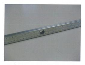
2) Insert silicone tube into the collared bush letting it protrude of minimum 5 mm per side:
