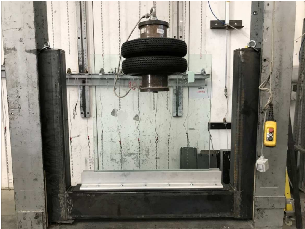
Photograph of the item after impact on the border of the glazing according to standard UNI EN 14019:2016
