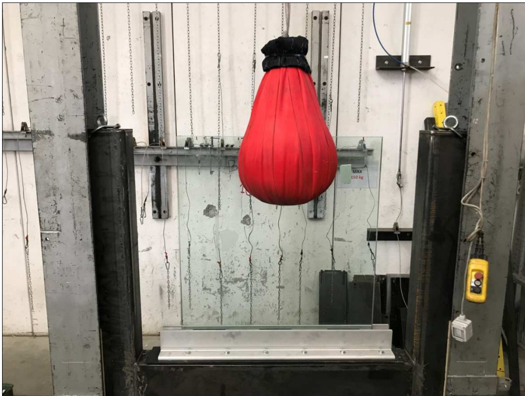
Photograph of the item after impact on the border of the glazing according to standard NF P01-013:1988
