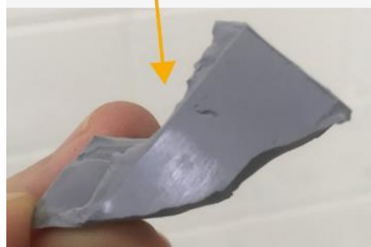
Figure 43: No adhesion on the inner side of the glass- Not OK
