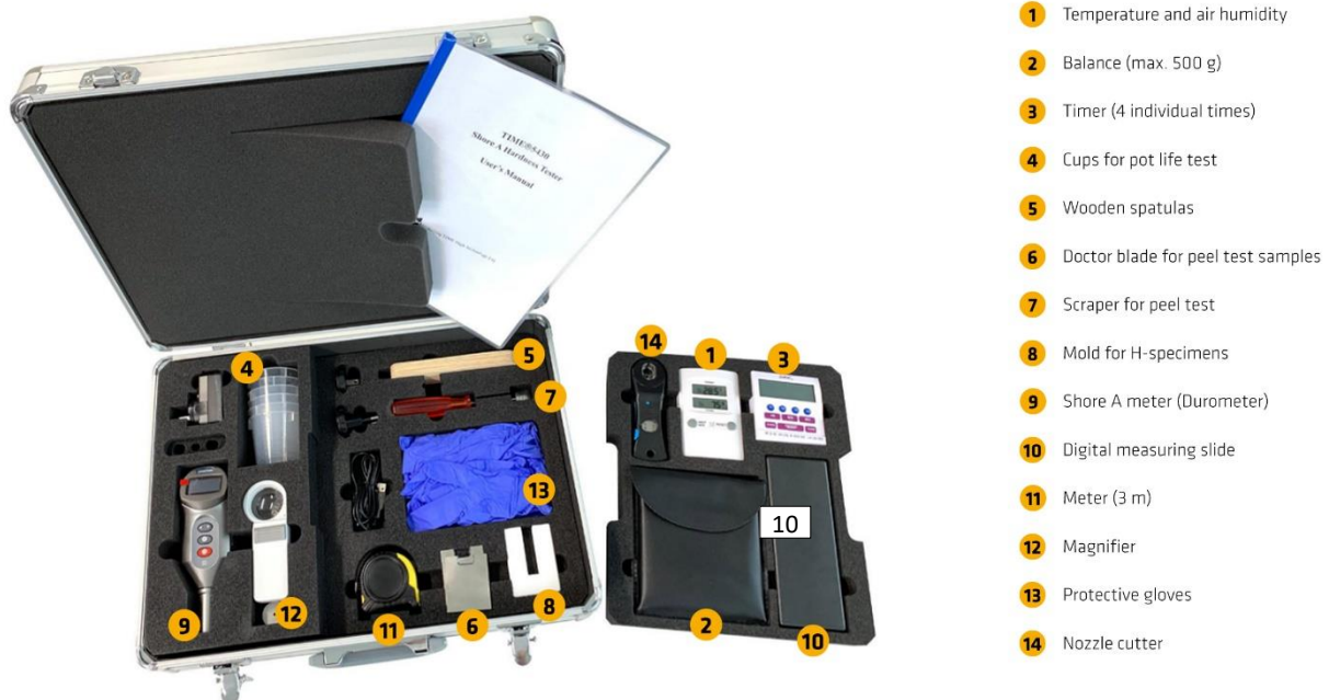
Figure 1: Pocket lab / Lab case for quality control
