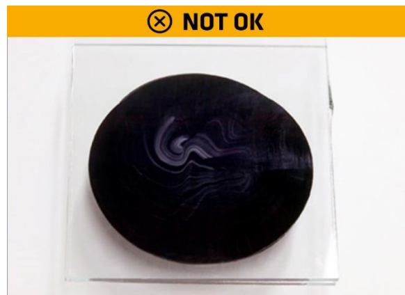
Figure 3: Negative test = inadequate mixing
