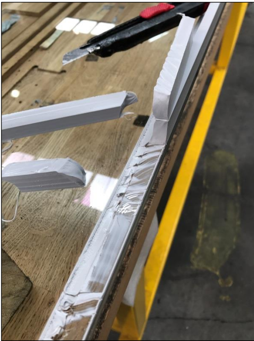
Figure 35: Good adhesion, deglazing test positive
