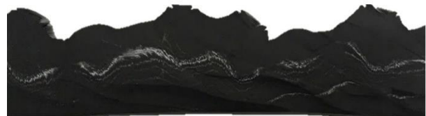
Figure 11: Severe white stripe in material, inhomogeneous mixing
