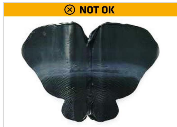
Figure 7: Unfold the foil - Negative test = inadequate mixing
