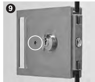
9/10) With a flat screwdriver fully tighten the screw inside its hole. During this operation you should see the button on the opposite side return inside the lock. Tighten fully.
