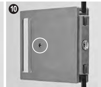
9/10) With a flat screwdriver fully tighten the screw inside its hole. During this operation you should see the button on the opposite side return inside the lock. Tighten fully.
