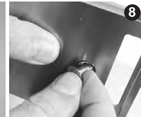
6) Take the internal cover and lean it against the internal plate. Make the 4 pivots of the cover coincide with the 4 holes on the plate. Then press the plate until the pins have been fully inserted.
